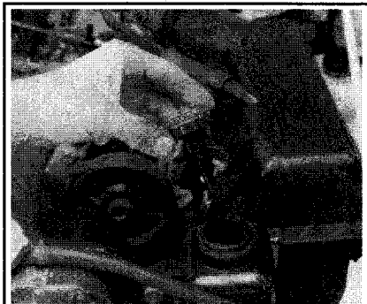
Fig. 127 Power steering fluid reservoir dipstick
